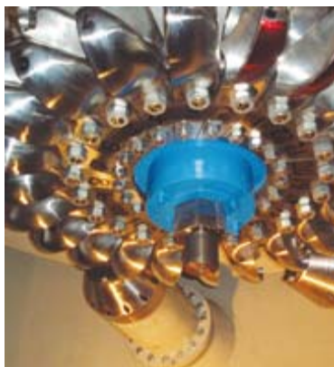
Pelton turbine with 6 nozzels
